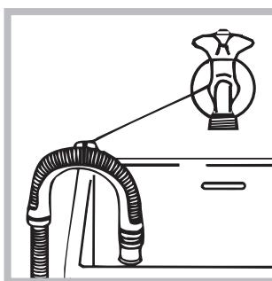
Alternatively, place the drain hose over the edge of a washbasin or bathtub, by fastening the guide (which can be purchased at the technical assistance centre) to the tap (see figure). The free end of the hose should not be underwater.
